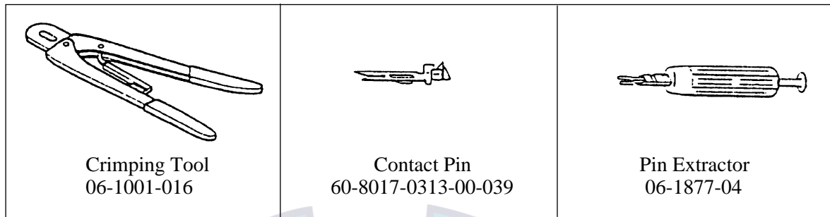
Figure 4-2a Crimping tool, contact pin, pin extractor
